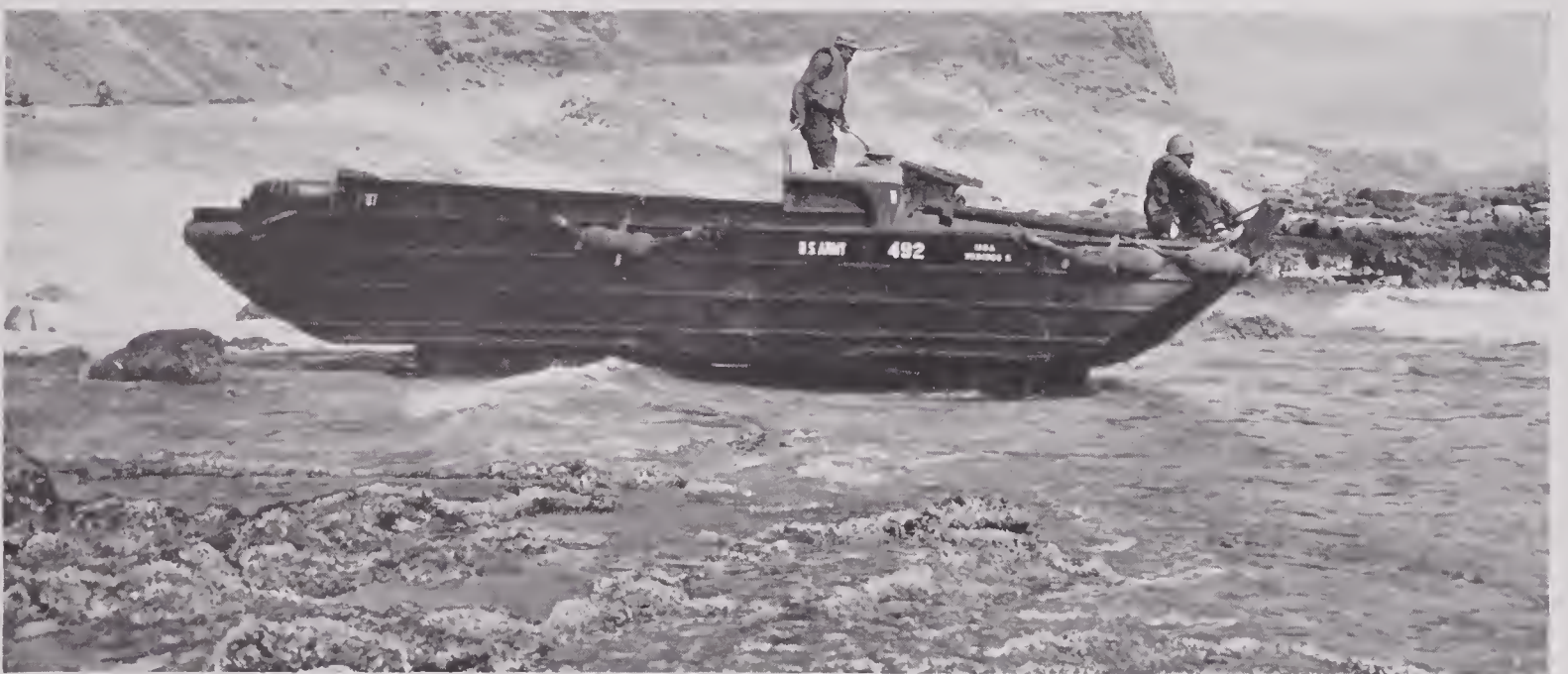
FIGURE 1. DUKW drivers training in coral driving techniques at Waimanalo. Lookout man is stationed on bow to select best route through bad reefs.
